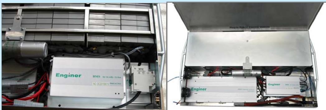
② **Connecting Mottcell Batteries:** Plug No.1-8 cell voltage wire into a socket marked with “L” on BMS; Plug No.9-16 cell voltage wire into the other socket marked with “R” on BMS.
